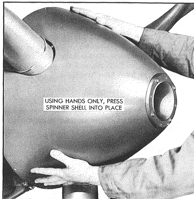
Figure 61—Installation of Spinner Shell
