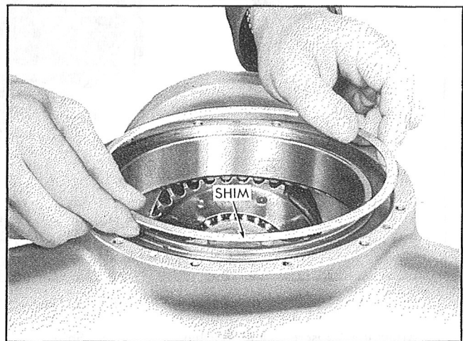
Figure 97—Removal of Shim
